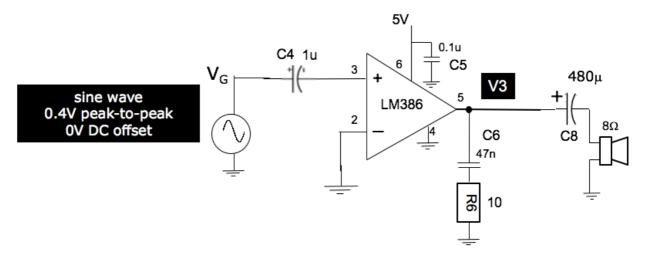
Instead of using the WG to generate sine wave signals, you can connect the input to the 3.5mm audio jack breakout board and supply the input signal using your phone via the 3.5mm audio cable provided. You now have a simple amplifier system that drives a speaker properly.
