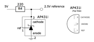
Modify the previous circuit by adding the 2.5V voltage reference as shown below, and verify that the gain of the amplifier is as expect. Why is this circuit an improvement from the previous version?
