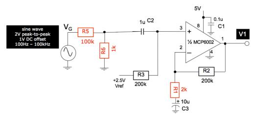
**Step 1**: Construct a voltage divider circuit with R5 and R6 as shown above. Generate a sine wave signal at 1kHz, 2Vpk-pk and 1Vdc offset. What do you expect to see at the input of the op-amp (i.e. pin 3)?
