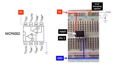
Insert a 0.1uF capacitor across the 5V and the GND rail as shown. This is called a "decoupling capacitor". It's function is to provide a very low impedance path for high frequency signals that somehow got onto the 5V power supply rail.
