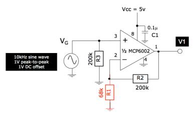
With the applied sine wave signal, measure the output  $V_1$  on the PicoScope. Record the waveform of  $V_1$ . What is the problem with this amplifier? Why does this happen and how might you fix this?
