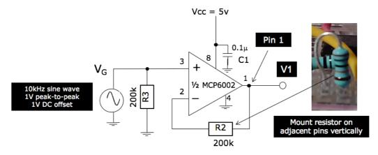
Now attached a 220 $\Omega$  resistor to Vo and comment on the loading effect with and without this op-amp.
