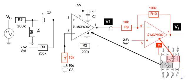
**Step 1:** Replace R1 with a 10k resistor. Use the second op-amp in the same package to construct the inverting amplifer and cascade your previous circuit (task 5). **What is the gain of stage one and stage two, and overall gain of the set up.** Verify this using the PicoScope and the WG.
